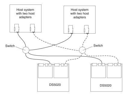
Figure 59. Example of two storage subsystems in a dual SAN environment
